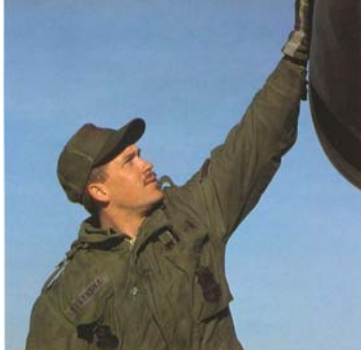
Top left Airman First Class Lukenbill, a flight line engine specialist, closes the cowling after completing his inspection of the No 3 engine of a B-52G of the 320th Bombardment Wing
